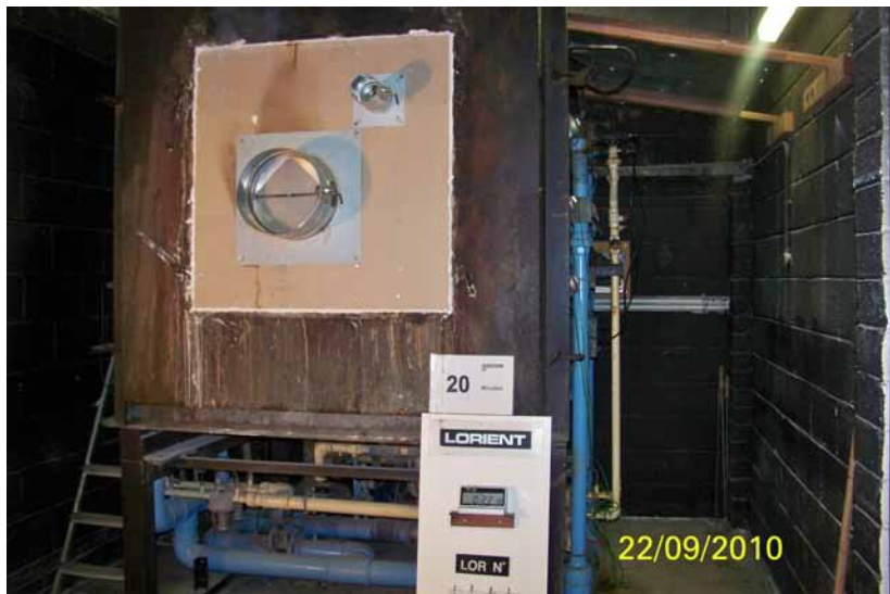
FTP 10 Fire test after 20 min's
