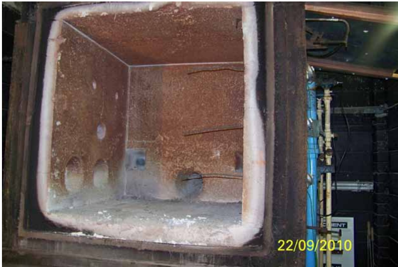
FTP 7 Internal view of furnace with front removed.
