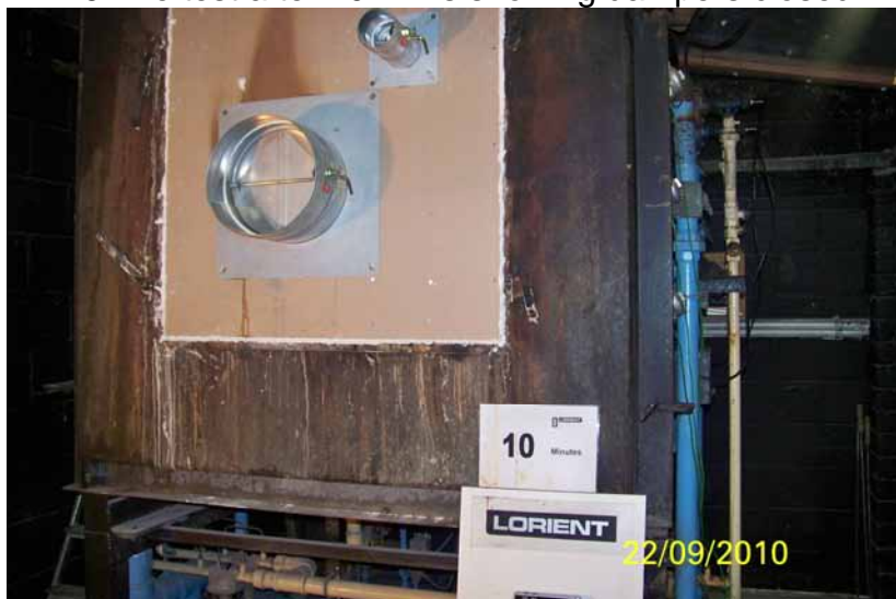
FTP 9 Fire test after 10 min's showing dampers closed.
