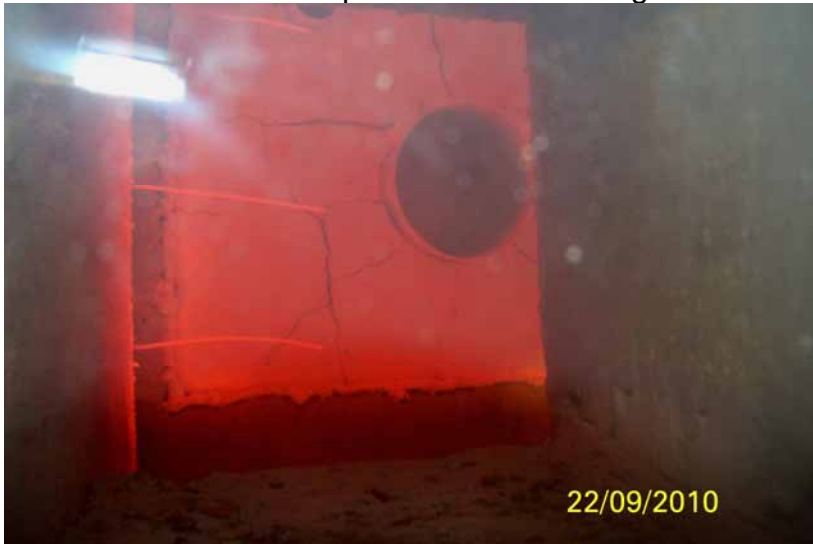
FTP 12 Internal view of plasterboard cracking at 25-30 min's
