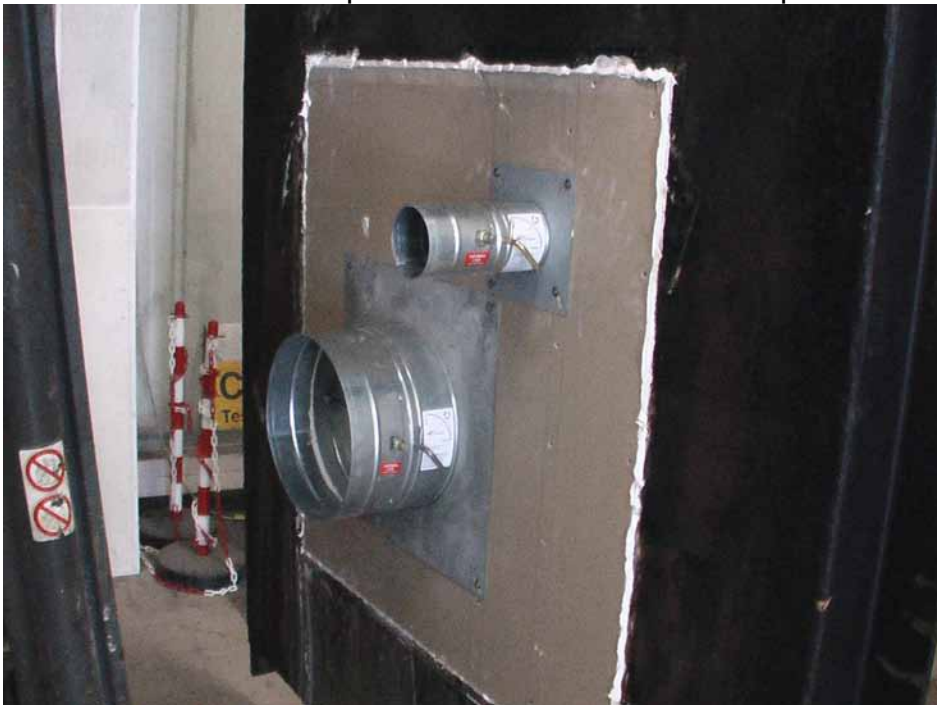
FTP 4 External face of specimen wall with Tri-Pro Dampers fitted.
