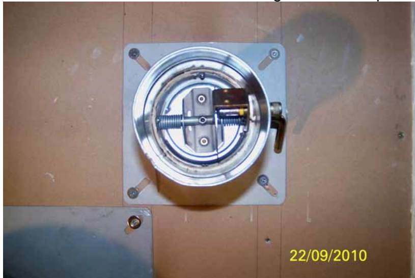
FTP15 Fire test after 45 min's showing 100 dia damper close up.
