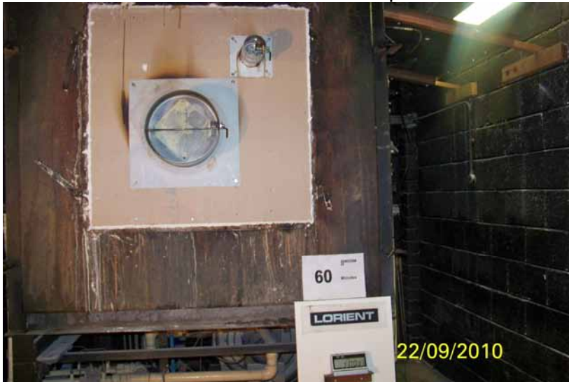
FTP18 After 60 min's the wall and damper are still demonstrating integrity.
